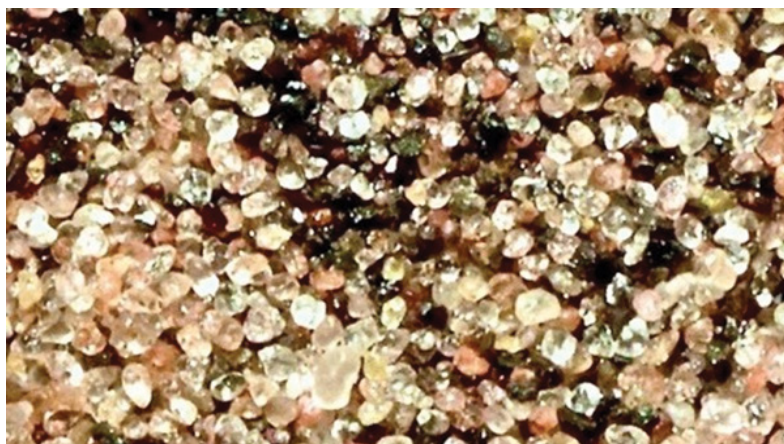
View of the well-rounded crystalline quartz sand optimal for fracking sand in the oil industry.
