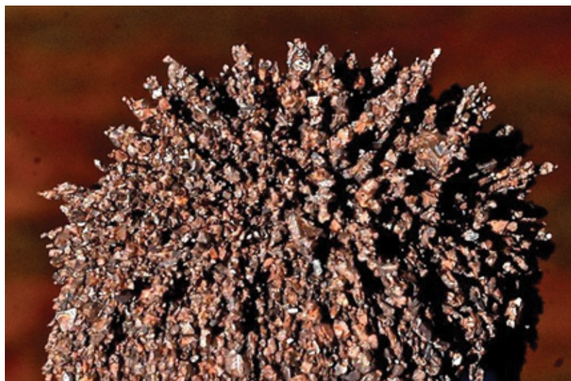
The main interest is the Ti-V magnetite, an easy commodity to separate by washing the clays.
