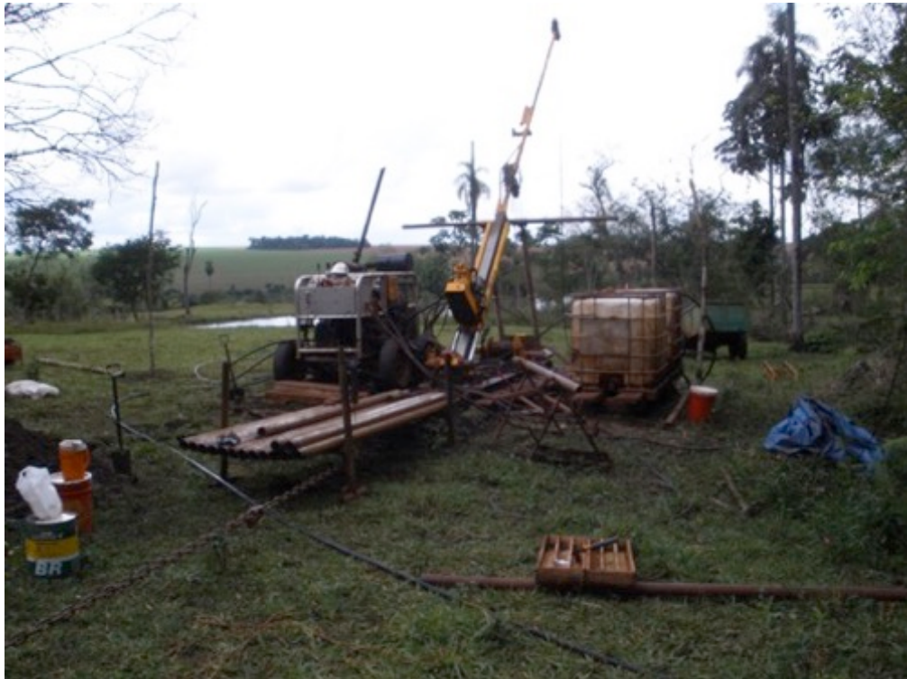
Deep auger and diamond drilling at the Itabo concession in 2007-2009
