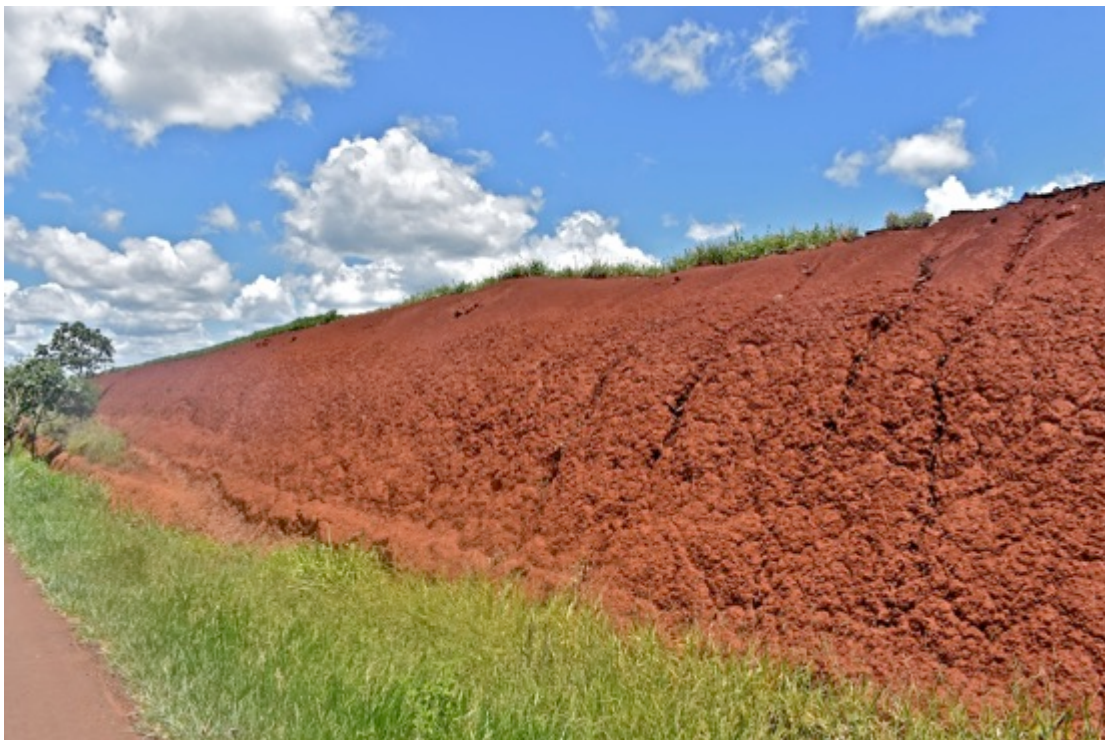
Laterites only outcrop along road cuts. View of outcrop several meters thick. XRF unit show similar values from top to bottom.
