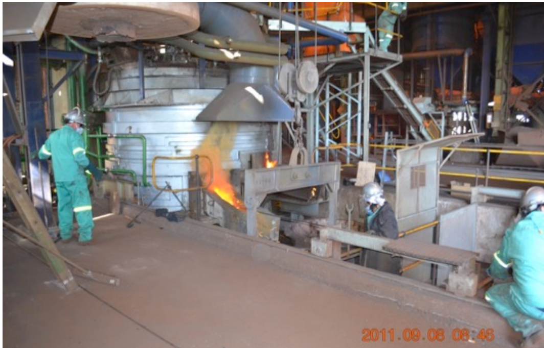
Lancing open the metal tap hole
