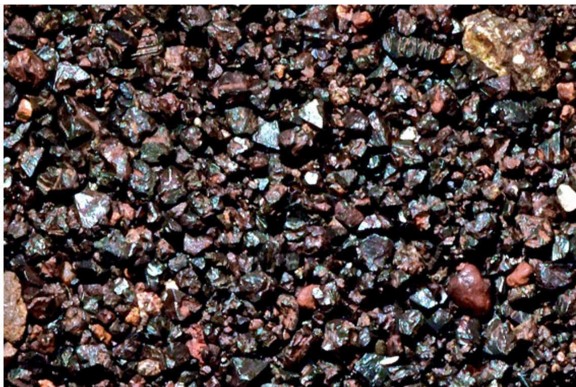
View of black sands in microscope show the octahedral Ti-V magnetite crystals.
